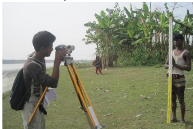
Figure: Embankment Cross section Survey
