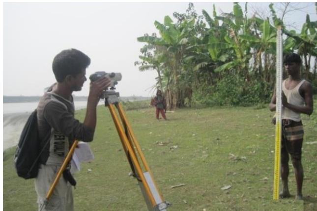
Figure: Embankment Cross section Survey
