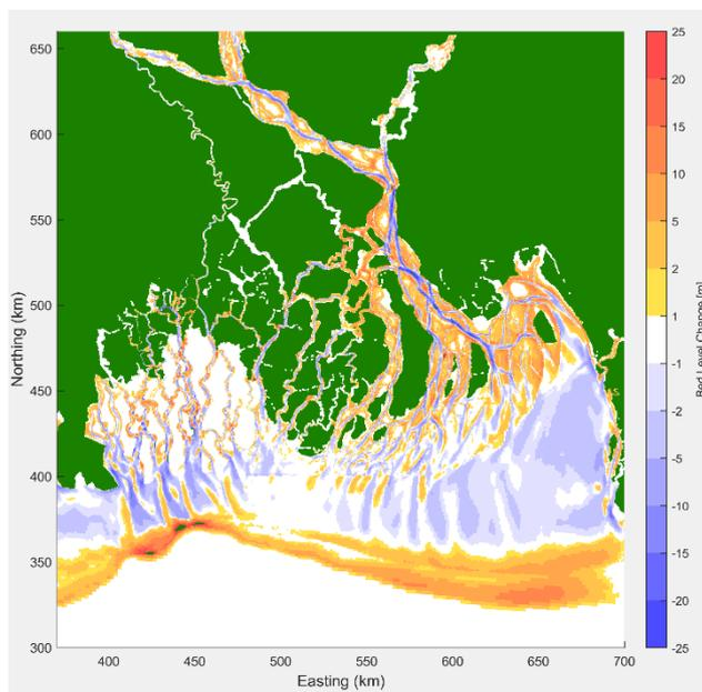
Figure 4.3 Simulated bed level changes, 2000-2019
