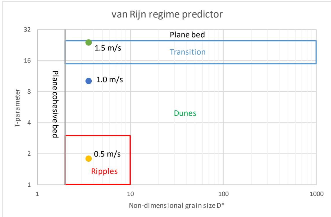
Figure 4.14 Application of the van Rijn regime predictor for the point bars in Pussur River.
