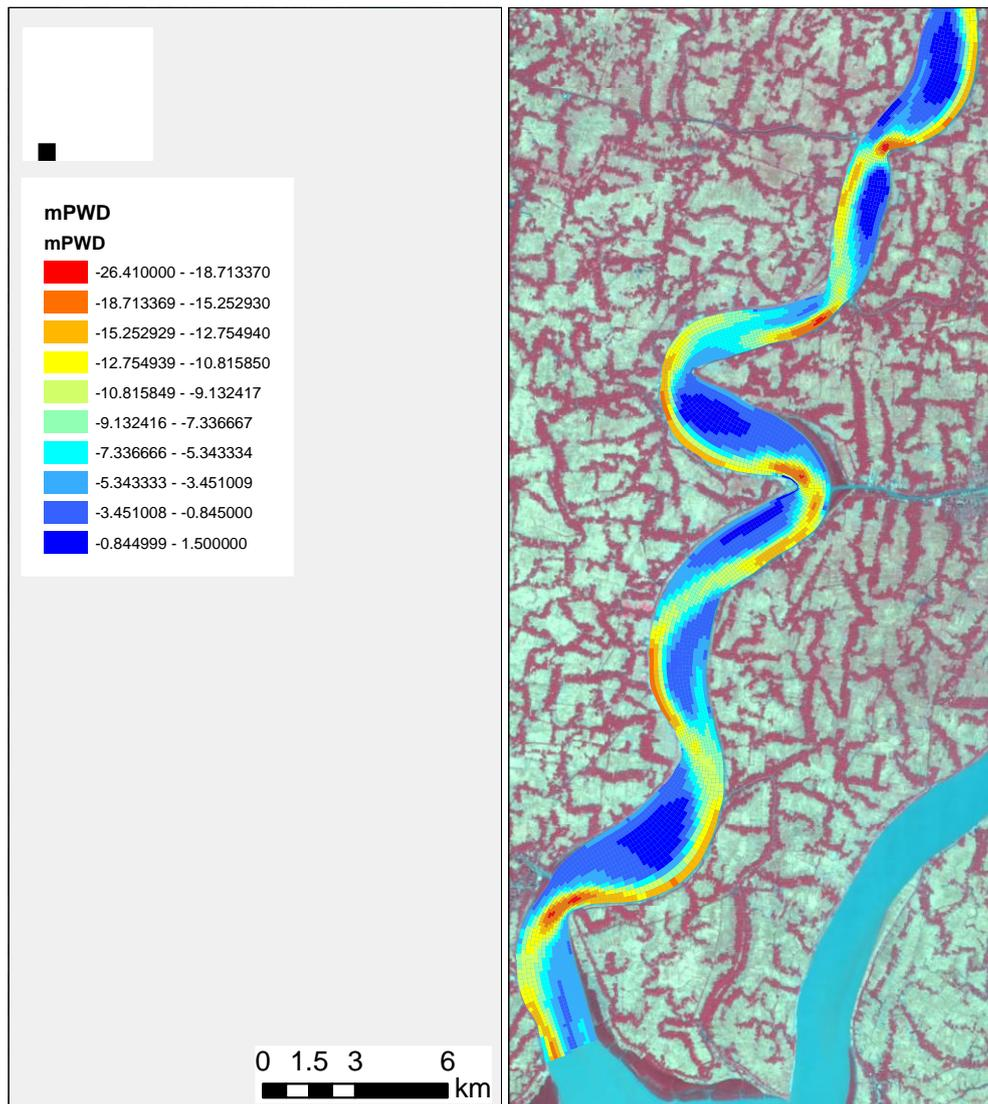
Figure 4.12 Bishkhali River model bathymetry based on the 2019 bathymetry data contoured to the 2019 grid.
