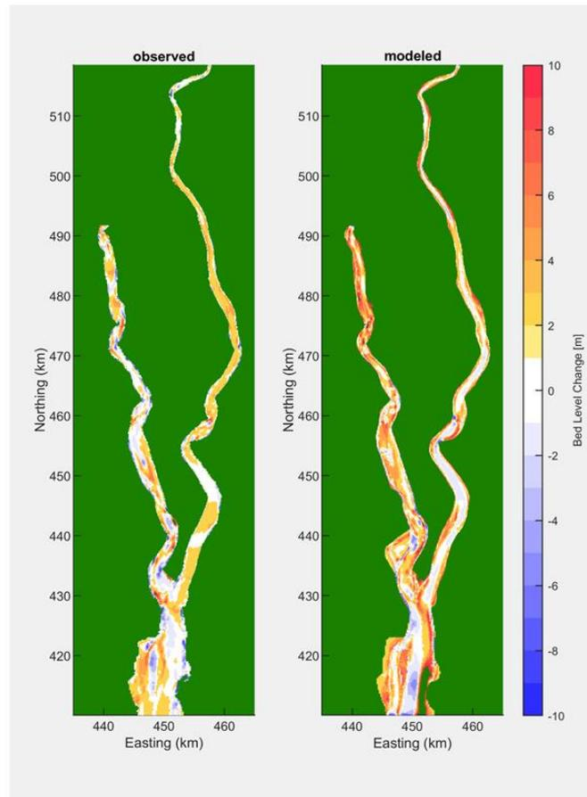
Figure 4.7 Sedimentation/erosion pattern after 9 years (2011 to 2019), measured (left panel) and modelled (right panel)
