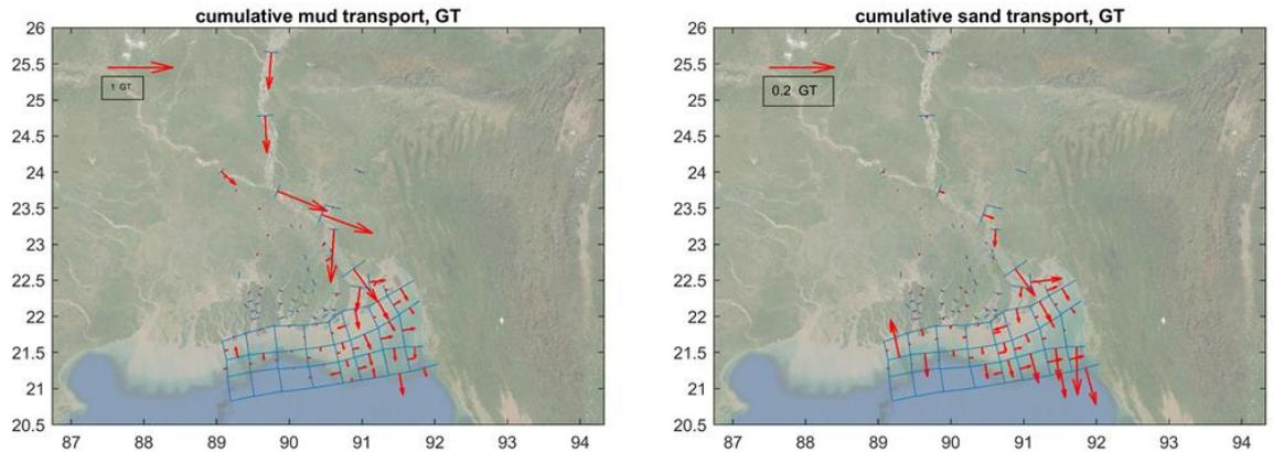
Figure 4.2 Yearly cumulative mud transports (left pane) and sand transports (right pane) in macro scale model, mind the different vector scales
