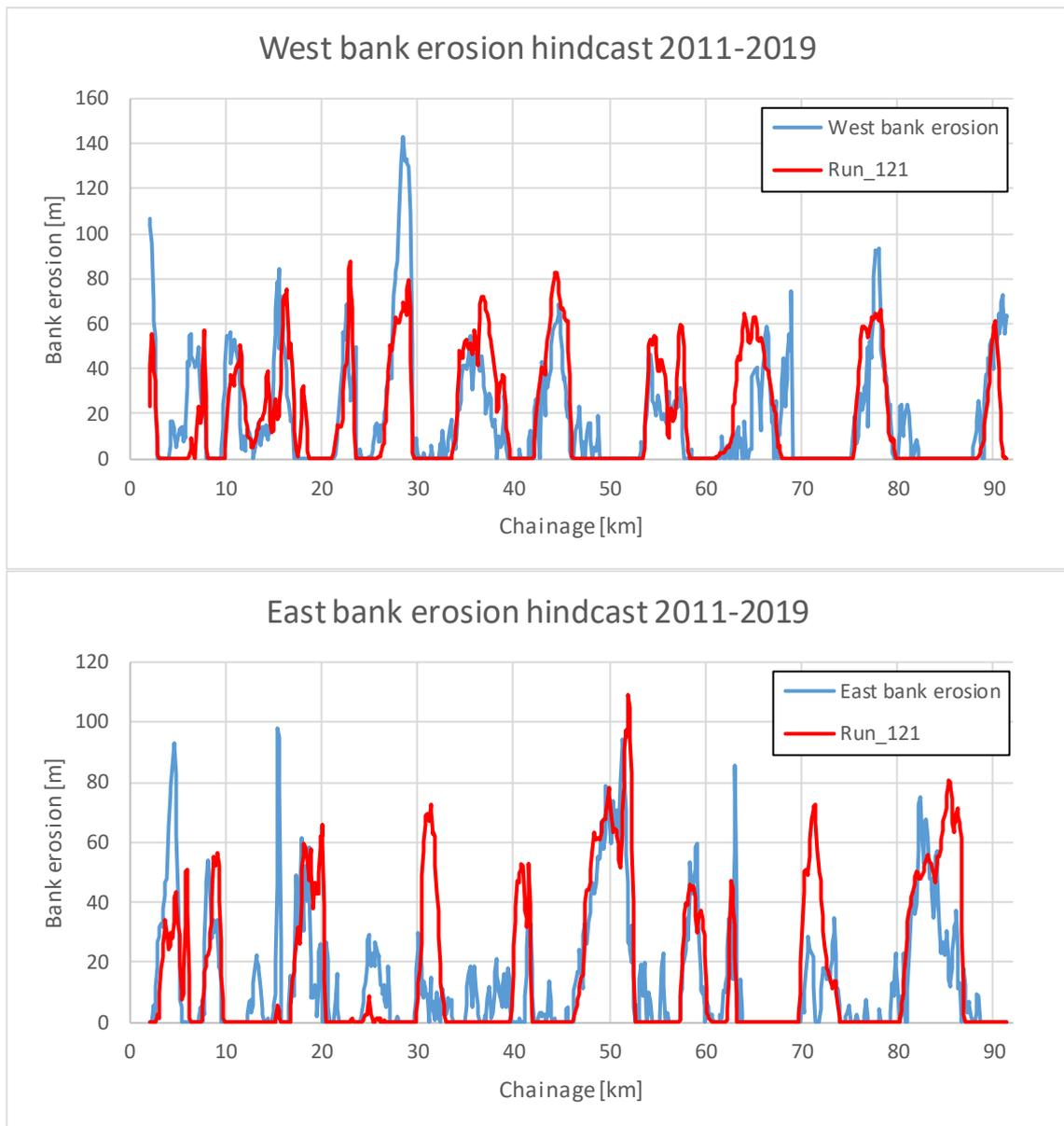
Figure 4.18 Observed and simulated bank erosion 2011-2019 comparison along the east and west bank of Bishkhali River.
