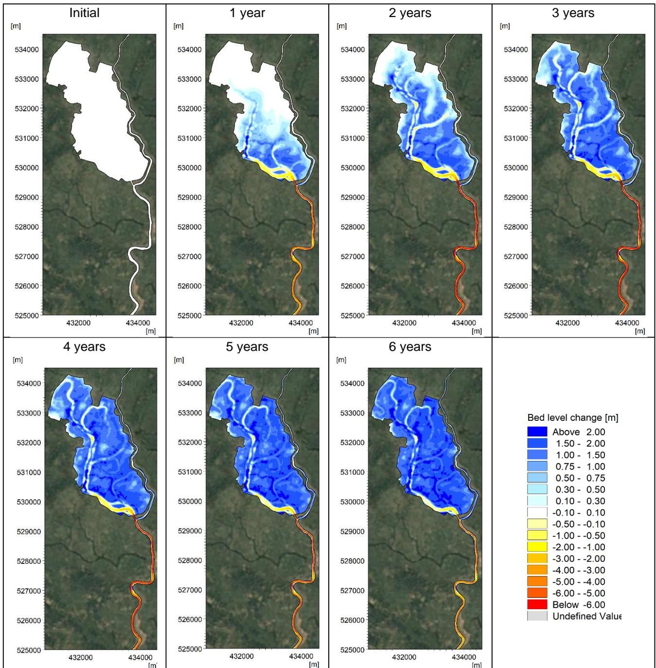
Figure 4.21 Bed level changes after activation of TRM at the southern end of the polder in the consecutive period of 6 years.
