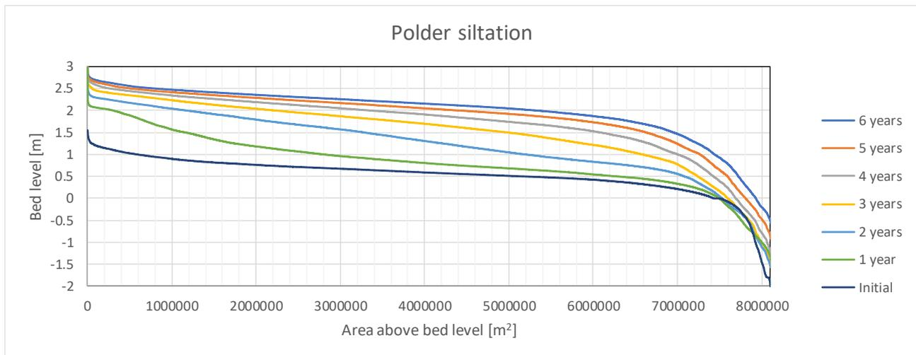
Figure 4.23 Area inside polder above a certain bed level during TRM operation.
