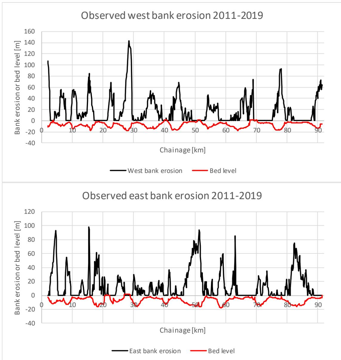
Figure 4.17 Observed bank erosion as function of chainage in Bishkhali River 2011-2019 for the east and west banks. The 2019 bed levels along the banks are shown as well to illustrate the strong correlation between bed levels and bank erosion, which we also see for Sibsa, Pussur and Baleswar. Note: We do not have a 2011 bathymetry for Bishkhali.
