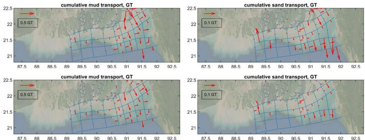
Figure 4.8 Yearly cumulative mud transports, details of (mind the different vector scales). Left panels are for mud. Top panels are with waves and wind. Lower panels are without waves and wind
