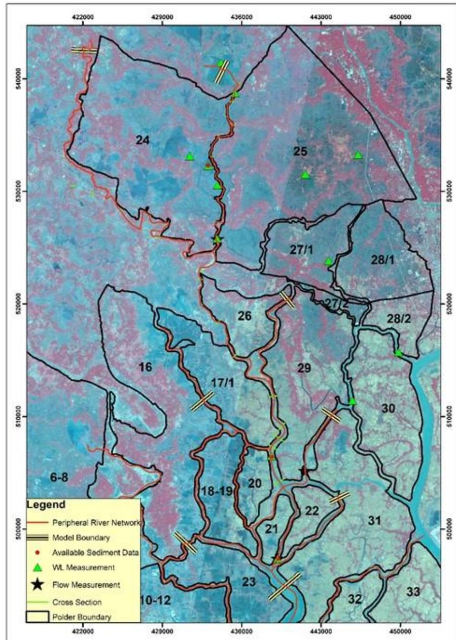
Figure 4.19 River Network for Mike 11 Model Extracted from SWRM
