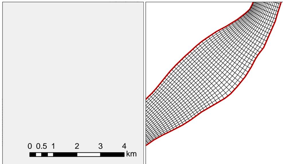
Figure 4.15 Illustration of the differences between the 2011 and 2019 grids, which cannot be identified without looking at the details. This is Baleswar, just upstream of the Gashiakali inflow where the eastern bank has been eroding consistently. The 2019 grid conforms to the 2019 bank line, as seen in the figure. The bank line moved roughly 100 m from 2011 to 2019.
