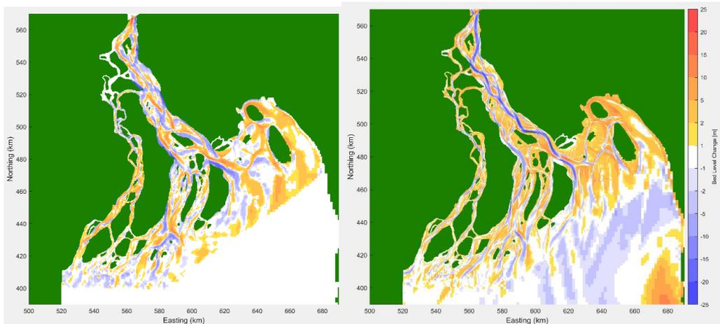
Figure 4.9 Observed (left panel) and simulated (right panel) bed level changes, 2000-2009, settings 2
