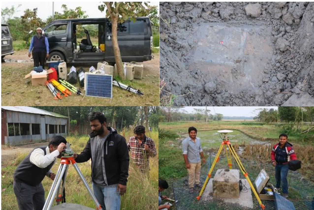
Figure 2.11: A). The suite of surveying equipment laid out in front of one of our vans and driver. B) close up of the buried monument at site 202. The brass pin with an X marking the measurement point is visible in the center of the concrete monument. C) Mondal and Sober using the tribrach and optical plummet on the tripod to center and level the antenna monument. D) Masud and Hasnat next to a completed station. The still open box holds the GPS receiver and power supply equipment. The solar panel is next to it, and everything is surrounded by a fence to keep the site from being disturbed.
