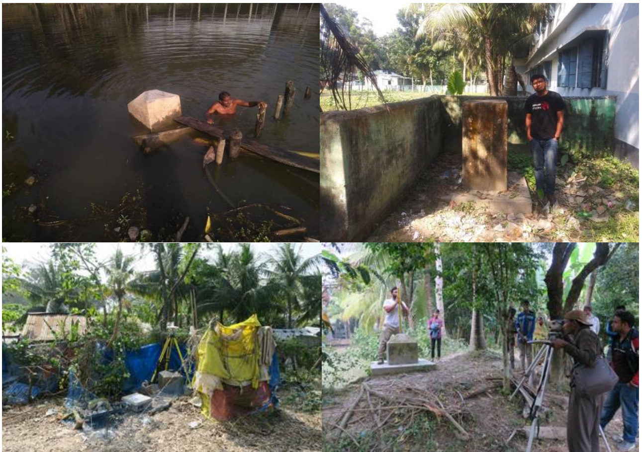
Figure 2.10: A). Monument GPS 198 was badly tilted and in the river. B) Example of a taller monument requiring a different tripod. The blocked sky view due to the building suggests that levelling to the monument would be best. C) Monument GPS 223 was surrounded by a squatter's home. However, with trimming trees and lowering the roof, we were able to obtain good measurements. D) Sober holds the survey rod while the IWM surveyor conducts a levelling line between the monument and the GPS system in the open field.
