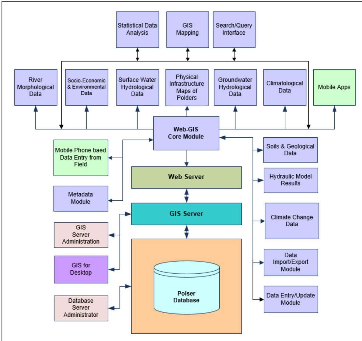
Figure 2-6: High-level System Architecture
