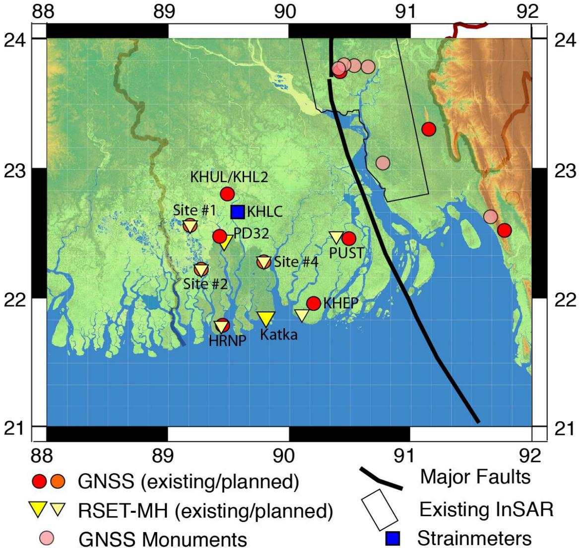
Figure 2-4: Locations of existing and planned GNSS and RSET-MH equipment in SW Bangladesh.
