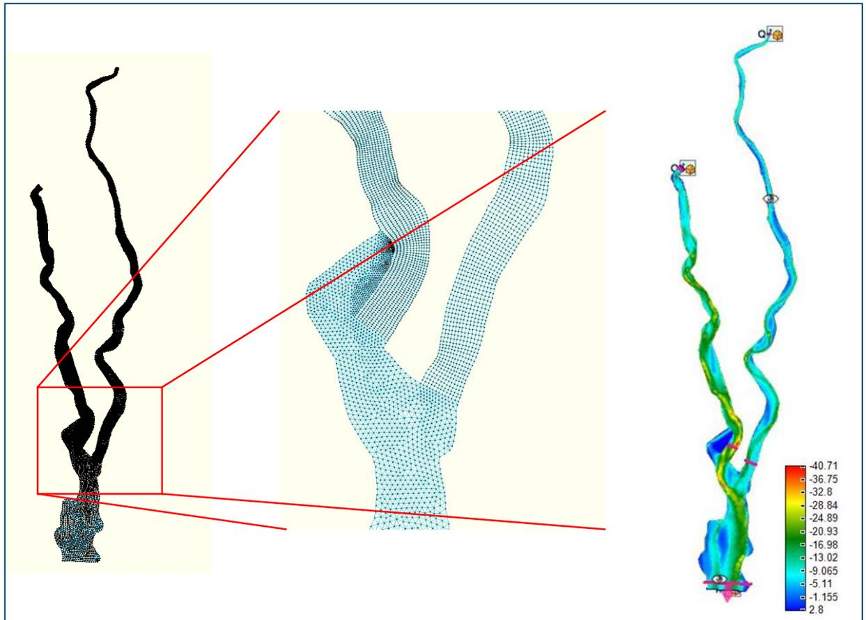
Figure 4-3: Computational mesh/grid for Pussur-Sibsa river system and interpolated bathymetry for 2011.
