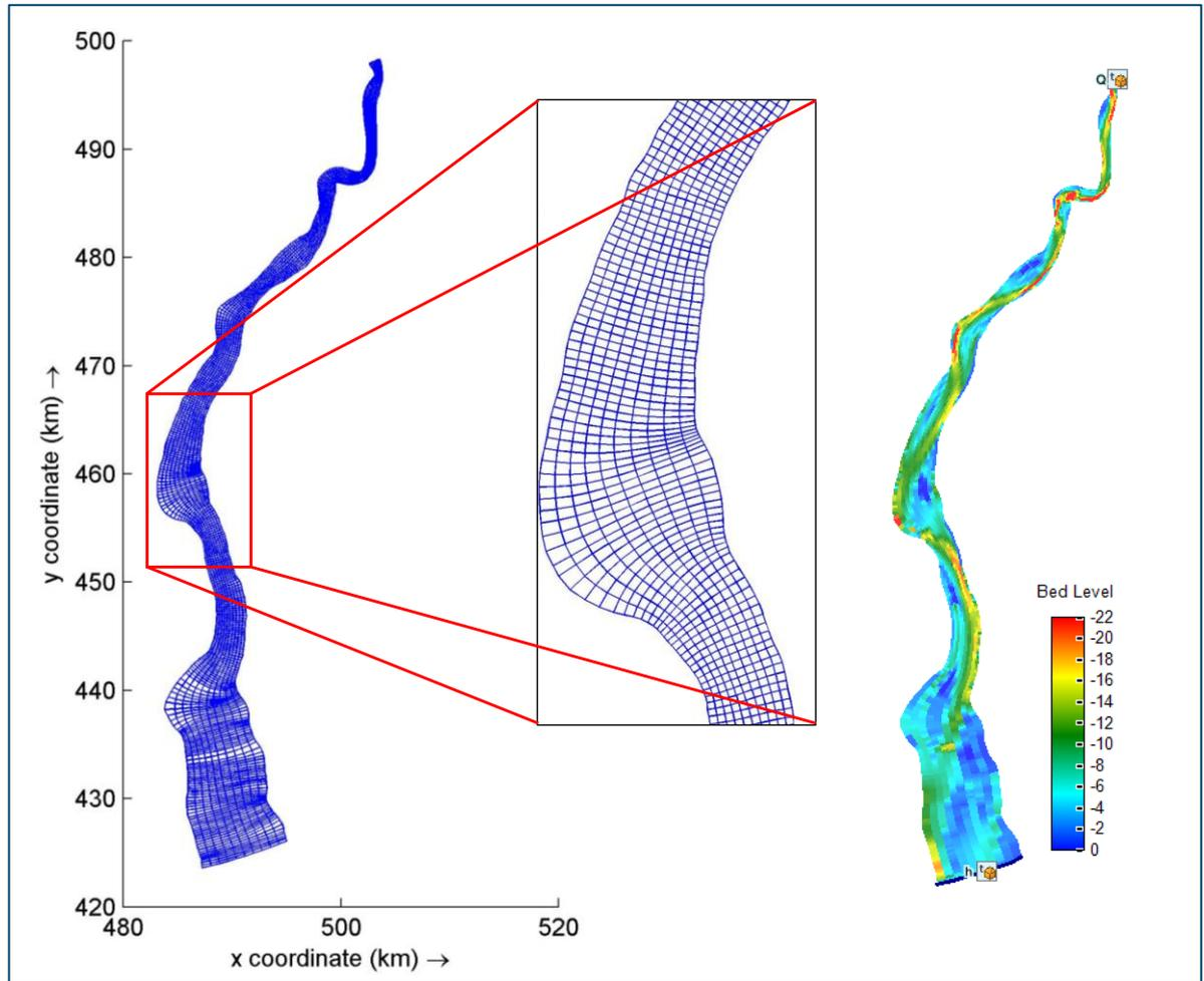
Figure 4-4: Computational mesh/grid for Baleswar river system and interpolated bathymetry for 2011.
