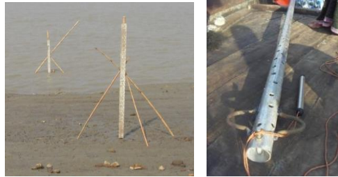
Figure 4.5 Water level gauge & Pressure Cell
