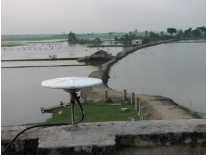
Photo-6: GPS measurements of Subsidence
