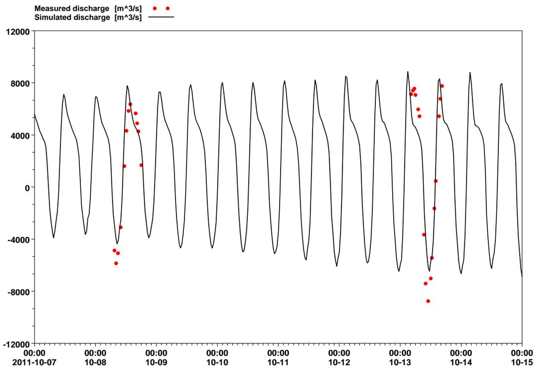
Figure 37 Discharge calibration at Mongla Port during Monsoon (ebb is positive, and flood is negative)
