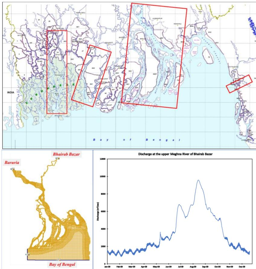
Boundary conditions and data for calibration and validation of models
