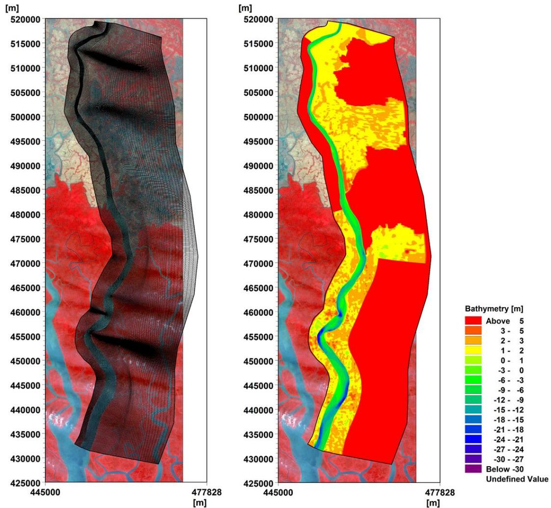
Figure 10 Computational curvilinear grid and interpolated bathymetry for the Pussur River.
