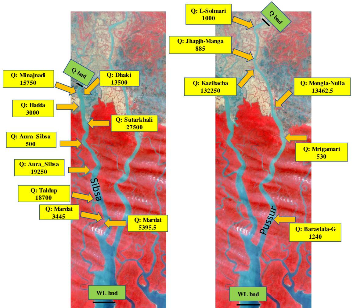
Figure 33 Boundaries location map in the Pussur-Sibsa river system. (yellow box indicate discharge from side channels from SWRM model chainage)
