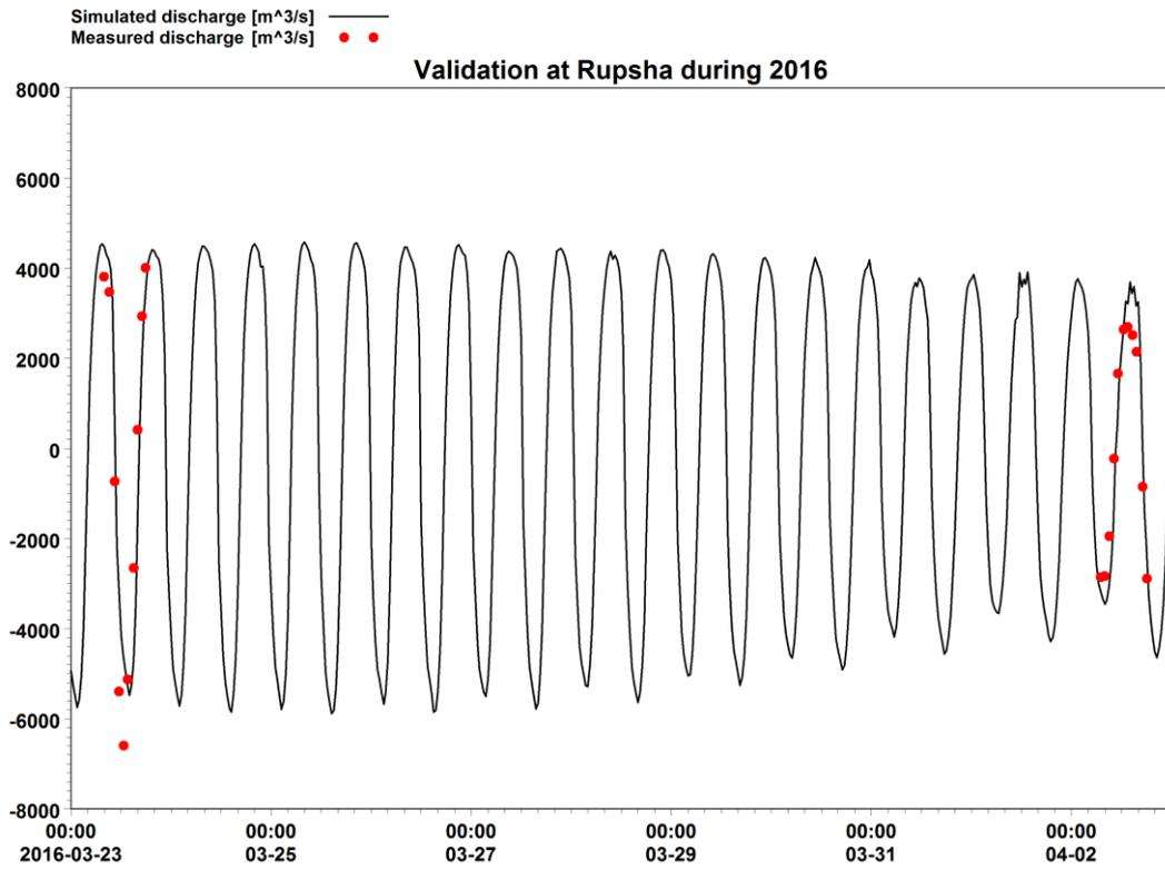
Figure 18 Discharge validation at Rupsha in Pussur river during 2016.
