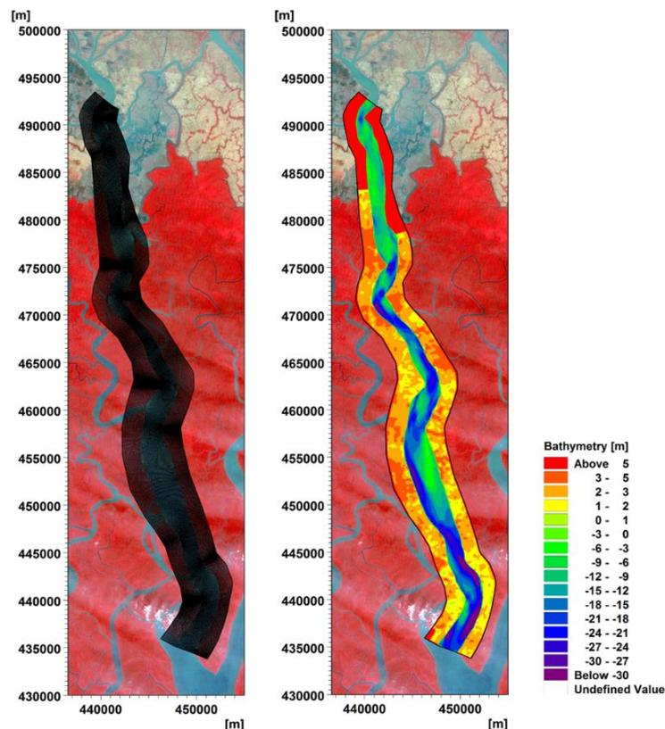
Figure 2 Computational curvilinear grid and interpolated bathymetry for the Sibs River. This version of the model includes floodplain and has a fine grid in the river channel (1000x30).
