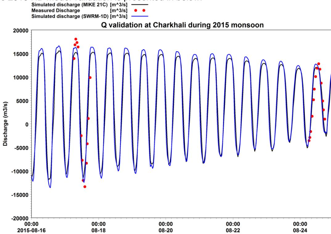
Figure 25 Discharge validation at Charkhali for 2015, also showing the SWRM 2015 results.
