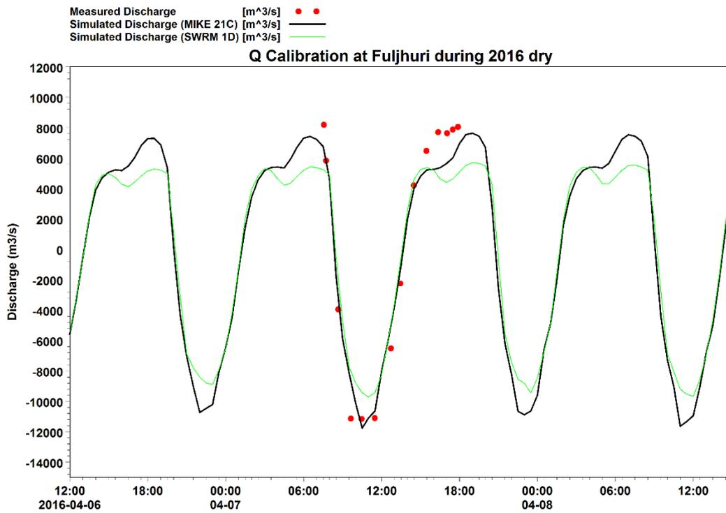
Figure 30 Discharge calibration at Fuljhuri during dry season (spring) for 2016.
