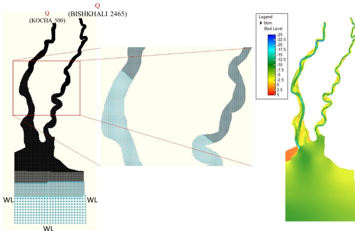
Figure 49 Computational mesh/grid (left panel) for Baleswar-Bishkhali river system and interpolated bathymetry (right panel) for 2019.
