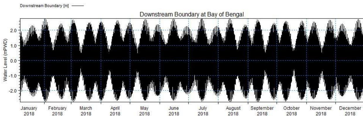
Figure 57 Downstream Water level Boundary of Sangu at Bay of Bengal
