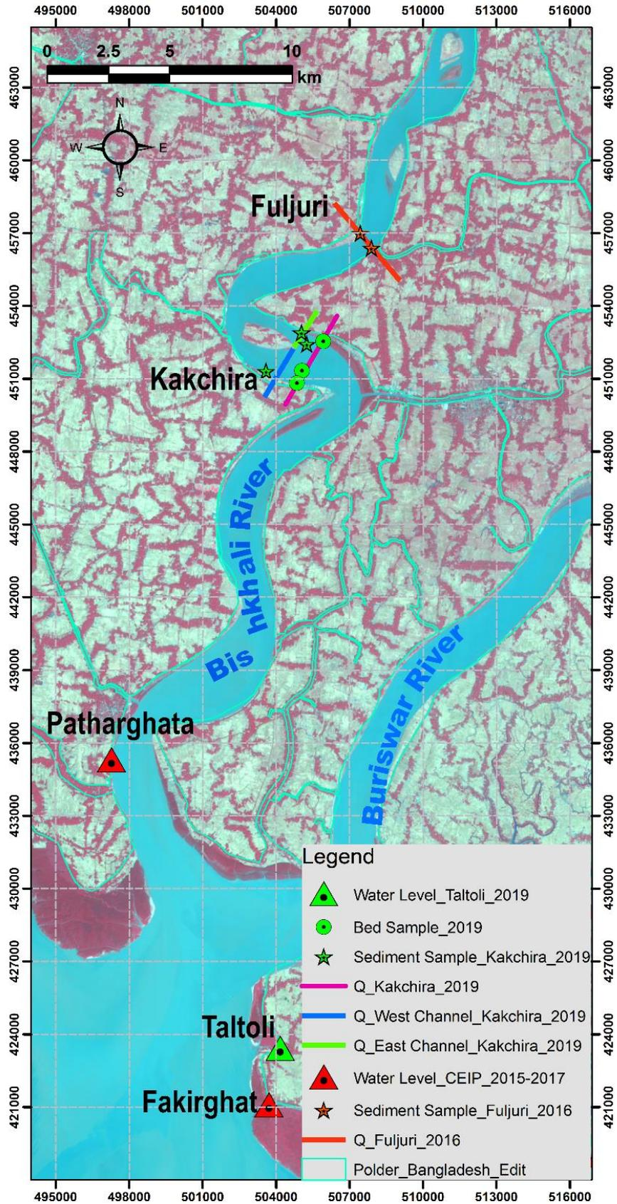
Figure 29 Discharge and water level Calibration (2016) and validation (2019) locations in Bishkhali River
