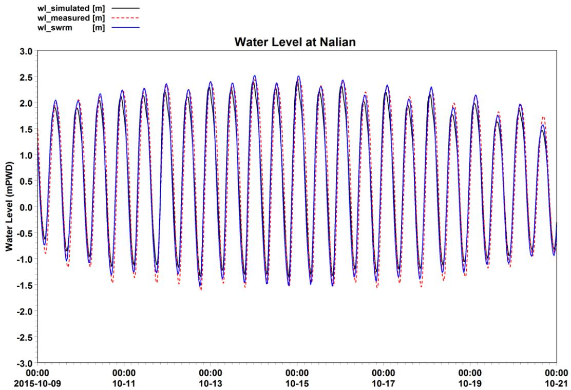
Figure 8 Water level validation at Nalian in Sibs River during 2015. The results include the Sibs model and the SWRM, and both validate convincingly against the Nalian water level observations.
