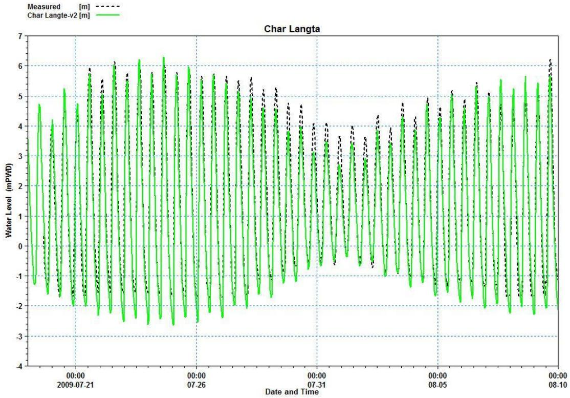
Figure 47 Water Level Calibration at Char Langta
