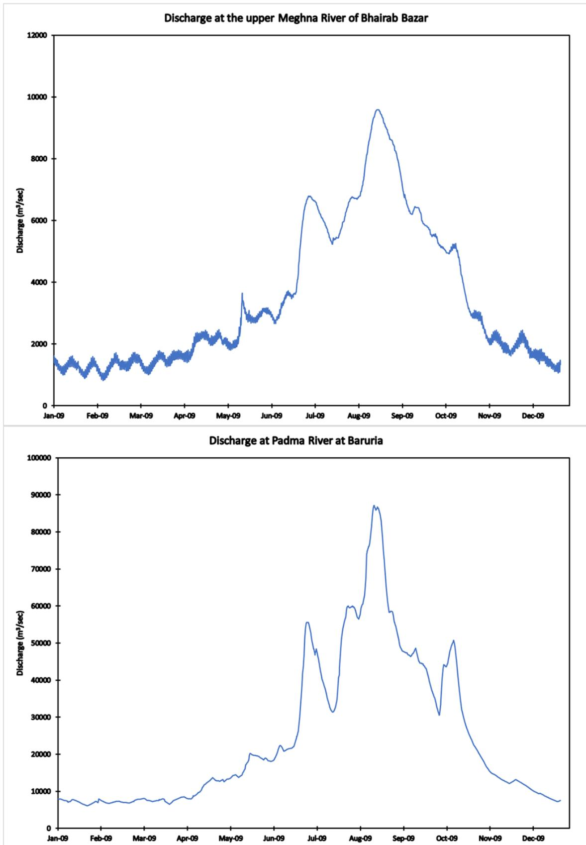
Figure 44 Discharge boundary at Bhairab Bazar of Upper Meghna River (upper panel) and Discharge boundary at Baruria of Padma River (bottom panel)
