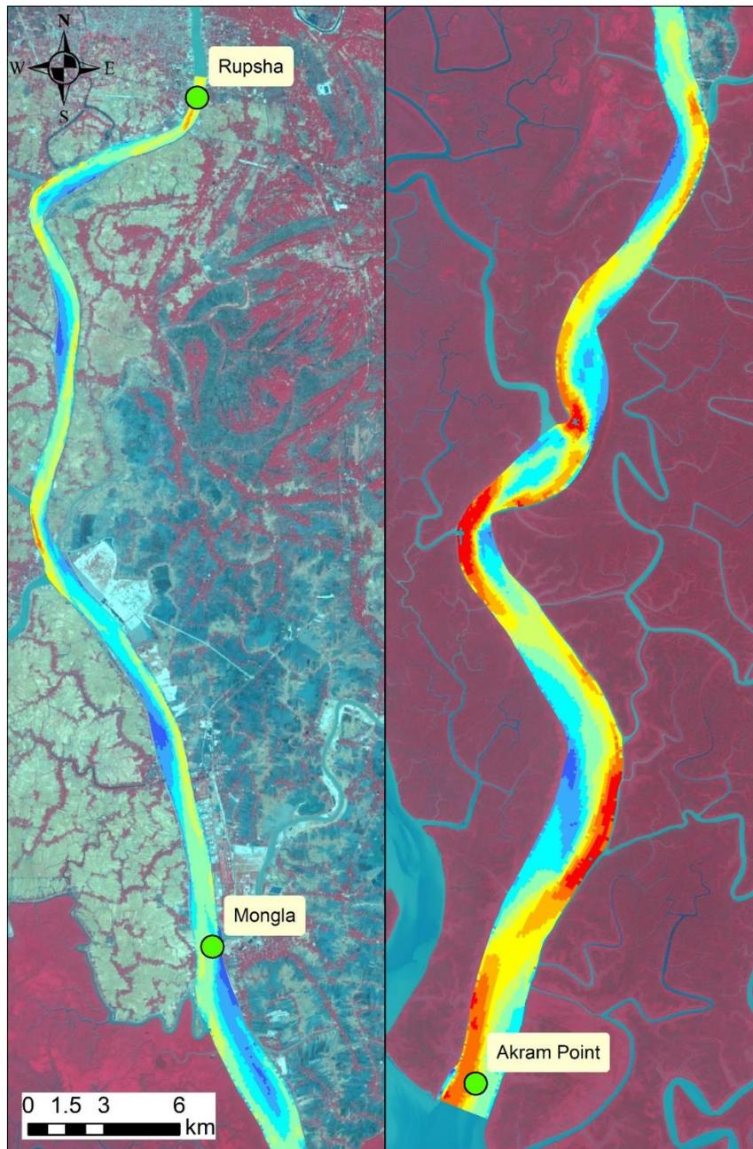
Figure 13 Field hydrometric data collection map for 2011. All three stations have discharge data, while only Mongla has water level data.
