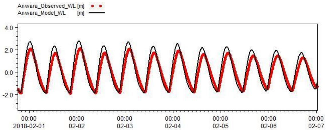
Figure 59 Water Level Calibration at Anwara (Dry 2018)
