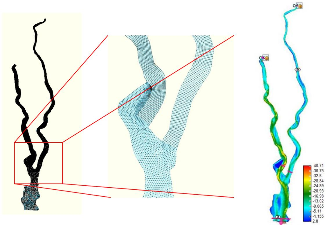
Figure 32 Computational mesh and interpolated bathymetry for the Pussur-Sibsa river system
