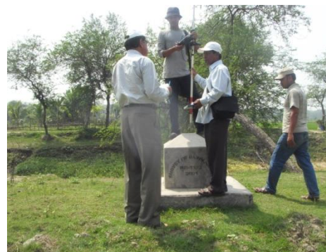
Figure 4.4: RTK GPS survey
