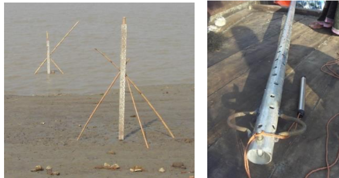
Figure 4.5 Water level gauge & Pressure Cell
