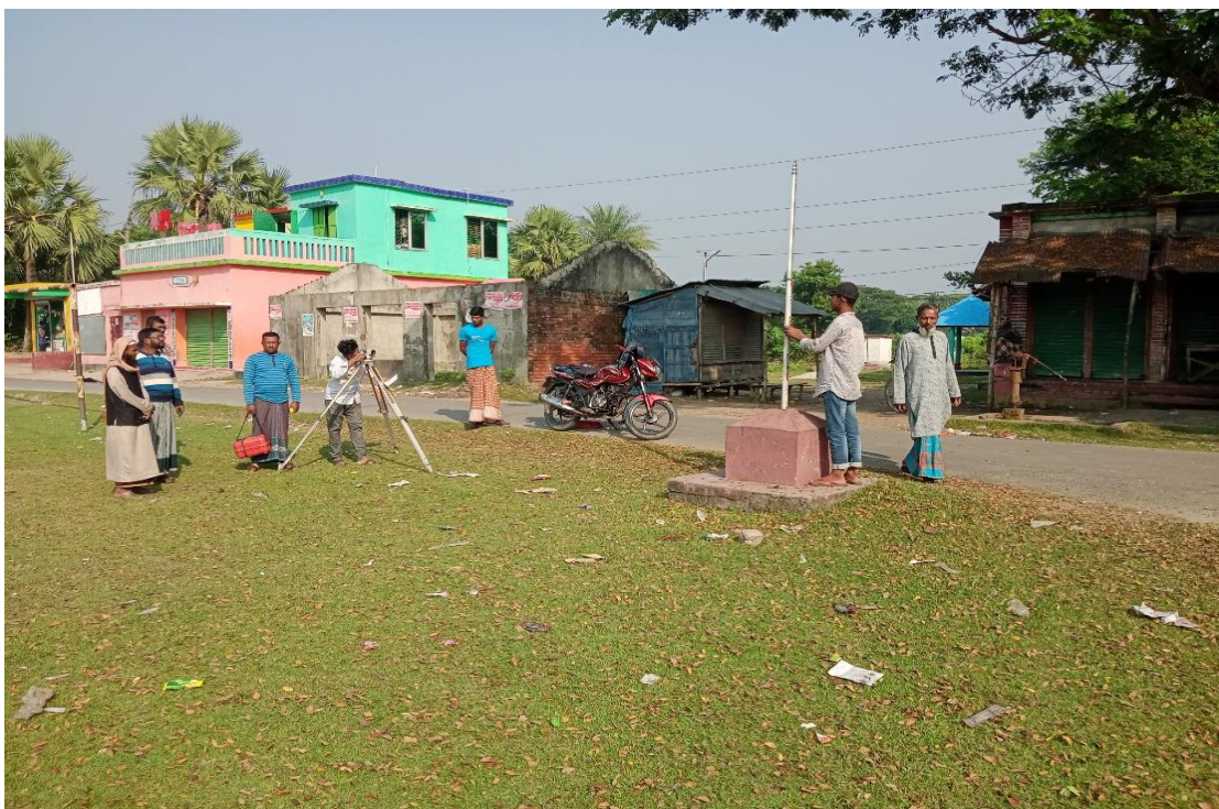
Figure 2-1: SOB Bench Mark at Dumuria, Khulna; used as reference to establish TBM for the Gangril and Badurgacha river sections
