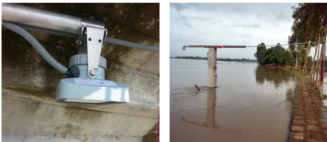
Figure 3-2: Sample Bridge mounted (left) and Pole mounted Structure (Right)
