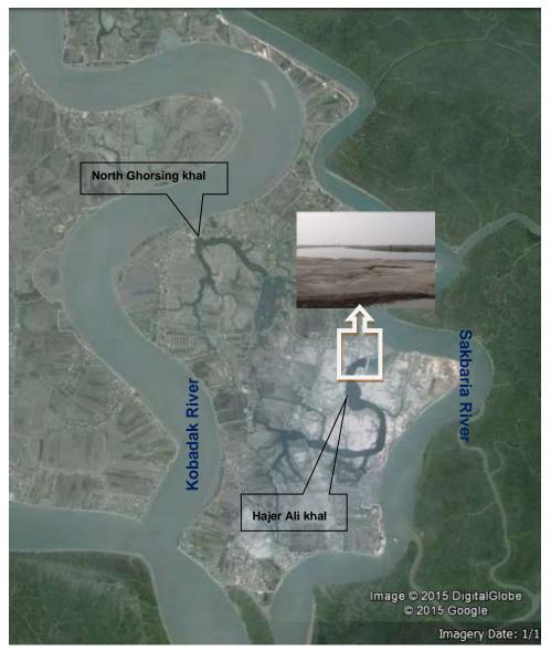
Figure 6.8: Extended Width of the Khals after Aila of the Polder 14/1
