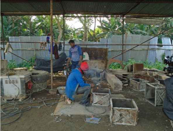
Workers welding work without using proper PPE at Badurtola Camp under polder no. 40/2
