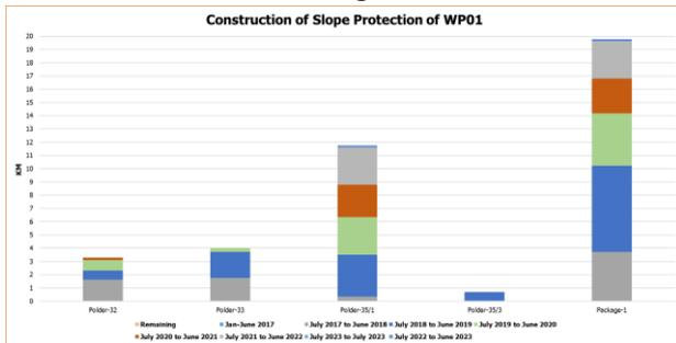
Figure 3-6: Construction of Slope Protection of Package-1
